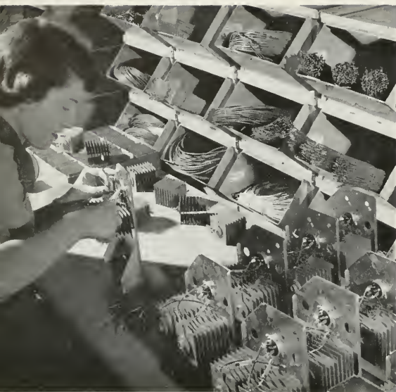
High voltage power supplies are assembled for use in new 21-inch RCA Victor color sets.
